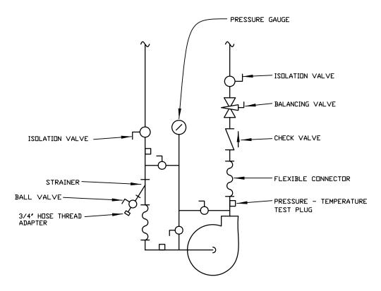
PROVIDE A MINIMUM OF 7 PIPE DIAMETERS OF STRAIGHT PIPE TO PUMP INLET. ALTERNATELY, PROVIDE SUCTION DIFFUSER IN PLACE OF STRAINER.
